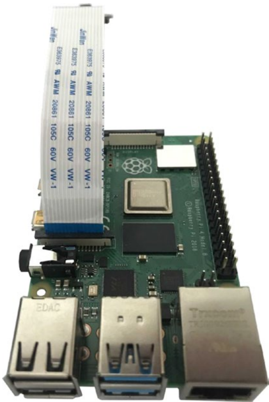
Figure 5-3. Camera module connected to the Raspberry Pi
